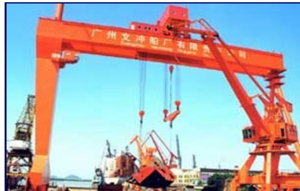
200 t Portal Crane
